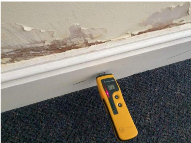
Damp meters, like this one, react to salt, and should not be used to diagnose rising damp.
